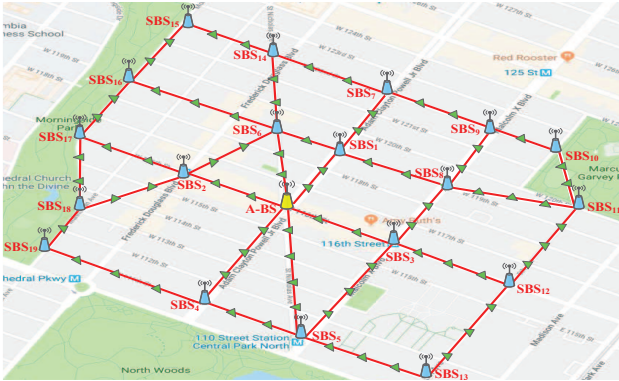
Figure 1: mmWave backhaul network model in a section of Manhattan.
