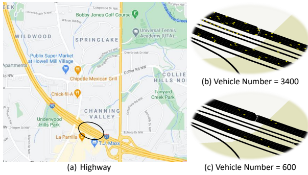
Fig. 2: (a) 3.5 mile highway section. (b), (c) are captured traffic images on the same 120m highway section. Each small yellow triangle represents a vehicle.
