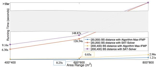
Fig. 7. Running times for SAT-solver and Alg. Max-IFMP
