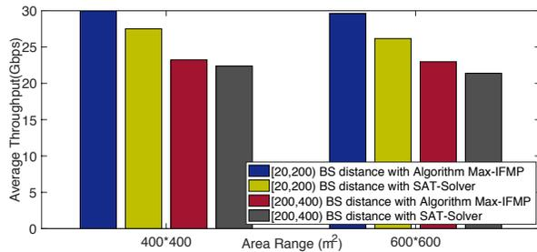
Fig. 8. Throughputs from SAT-solver and Alg. Max-IFMP
