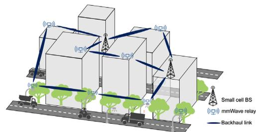
Fig. 1. Multipath Construction in Relay Assisted mmWave Backhaul Network
