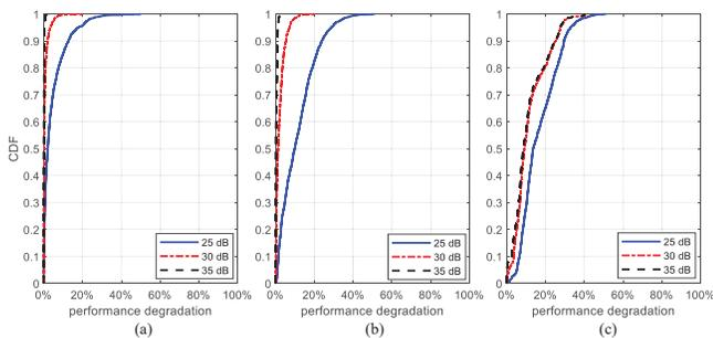
Fig. 9. Throughput performance degradation with more accurate interference model for different main beam to side lobe ratios ( $l_g = 300$  m,  $B = 15^\circ$ )
