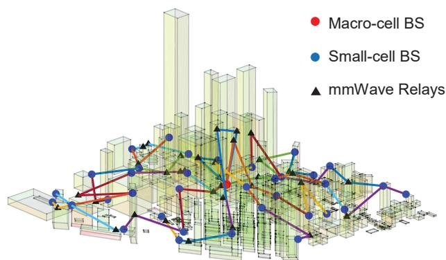
Fig. 1. A relay assisted mmWave backhaul network in downtown Atlanta.
