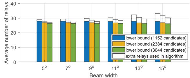
Fig. 8. The number of relays used ( $l_g = 300 \text{ m}$ )
